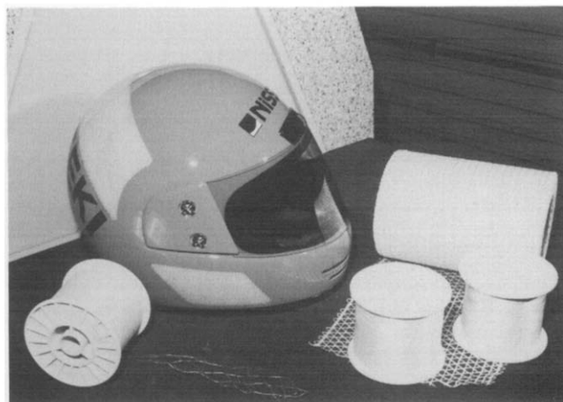
Figure 6 High-strength high-modulus polyethylene tape, yarn and fabric; helmet is yarn with epoxy
